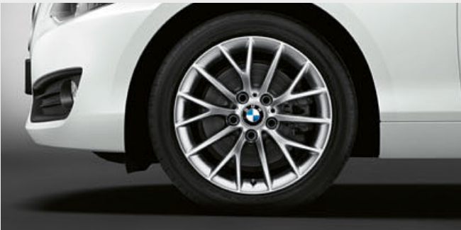
□ 17" light alloy wheels Y-spoke style 380, 7J x 17 with 205/50 R17 tyres.
