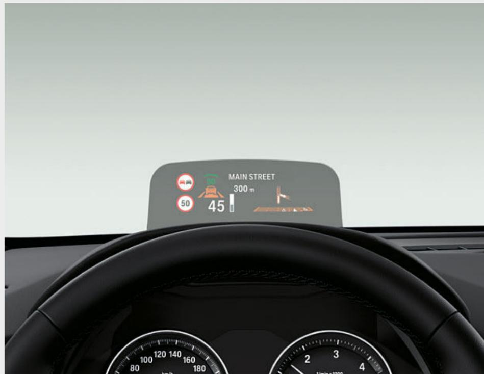
□ The full-colour BMW Head-Up Display<sup>1,8</sup> projects all relevant driving information onto a panel in the driver's field of vision, which means they can remain focused on the road. Current speed, directions from the navigation system, Speed Limit Info incl. no-overtaking indicator and telephone and entertainment lists, among other things are displayed.
