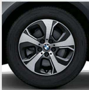
□ 16" light alloy wheels turbine styling 472<sup>1,2</sup>, BMW EfficientDynamics, Orbit Grey, gloss-lathed, wheel size 7J x 16, 205/60 R16 tyres.
