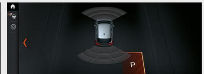
□ The Parking Assistant<sup>8</sup> makes parallel parking easier. The system works by measuring potential spaces while driving past them at a low speed. When a suitable space has been found, the Parking Assistant takes over steering, while you are responsible for selecting the correct gear, as well as pressing the accelerator and brake.
