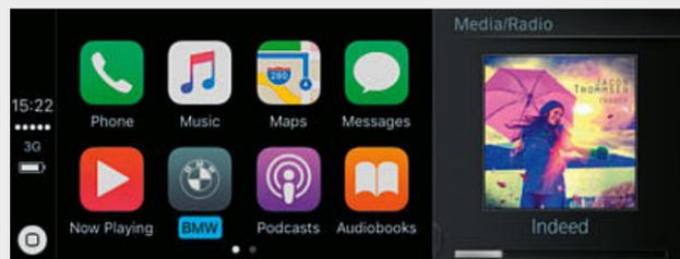
□ Preparation<sup>5,6</sup> for Apple CarPlay<sup>®</sup> supports the convenient and wireless use of selected iPhone<sup>®</sup> functions in the vehicle. This allows smartphone content and functions such as music, iMessages/text messages, telephony, Siri, navigation and selected third-party apps to be displayed and operated via the vehicle's user interface and via Voice control.
