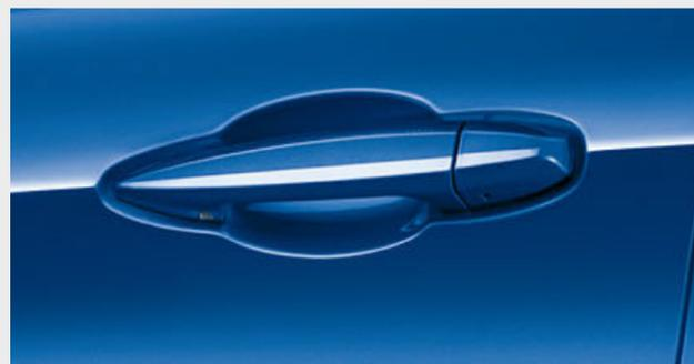
□ The Comfort access system allows passengers to enter the car via the front doors and to open the tailgate without having to actively use the key. The key must simply be nearby, in the driver's trouser pocket for example. To unlock the doors, it is only necessary to touch the handles or the tailgate button.
