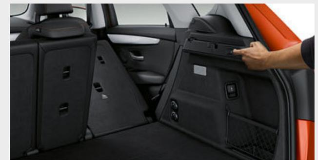
□ Remote backrest unlocking for the rear seats<sup>7</sup> allows the rear seat backrests to be unlocked and folded down conveniently via a button in the luggage compartment.
