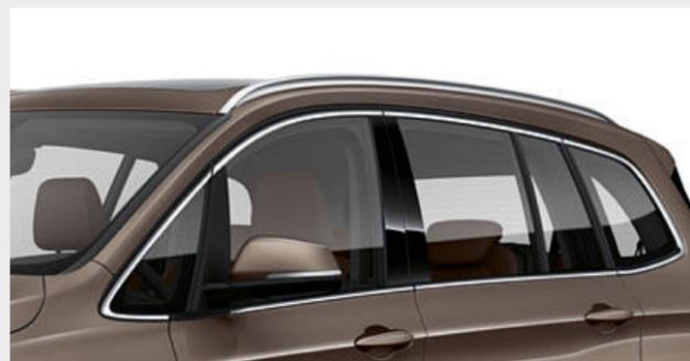
□ The Roof rails in Aluminium satinated provide the base for a multifunctional BMW roof rack unit.
