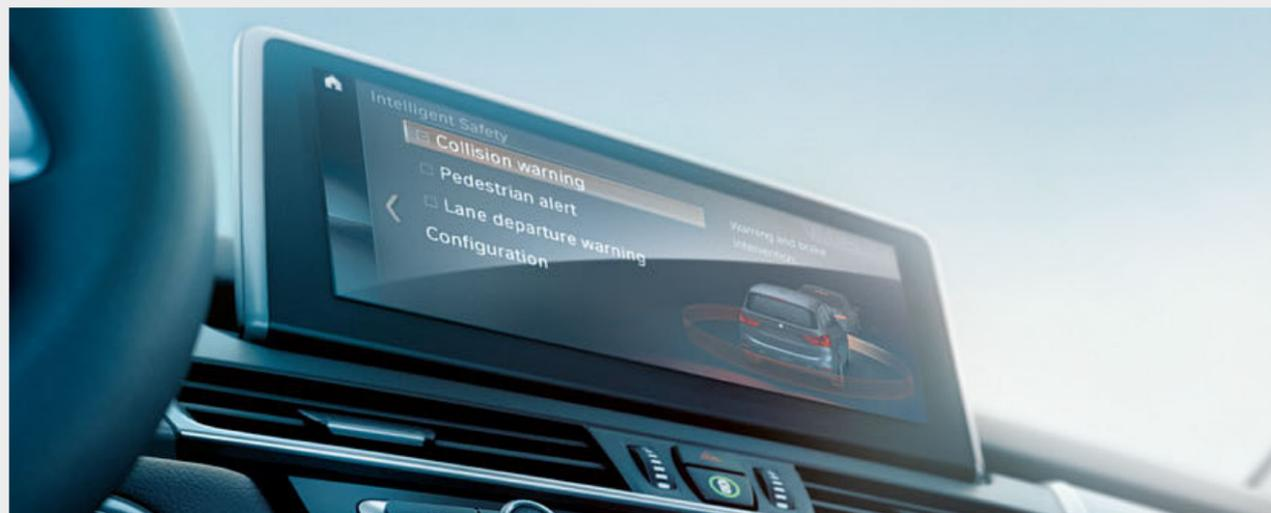
The safety package **Driving Assistant**<sup>1,2,5</sup> includes camera-based assistance systems, such as Lane Departure Warning, Approach control warning, High-beam assistant and Speed Limit Info. The Approach control warning and Person warning with light city braking function warns of collisions at speeds between 10 and 60 km/h, while the Lane Departure Warning causes the steering wheel to vibrate as a warning when the lane is unintentionally changed at 70 km/h or over.
