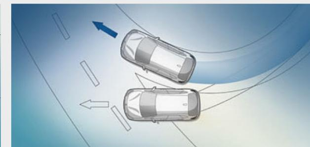
■ **Dynamic Stability Control (DSC)** continuously assesses the vehicle's movements using various sensors and stabilises the car with engine and braking regulation when unstable driving conditions are detected. Auxiliary functions include braking readiness, brake drying by the braking system in wet conditions and the Hill-Start assistant.
