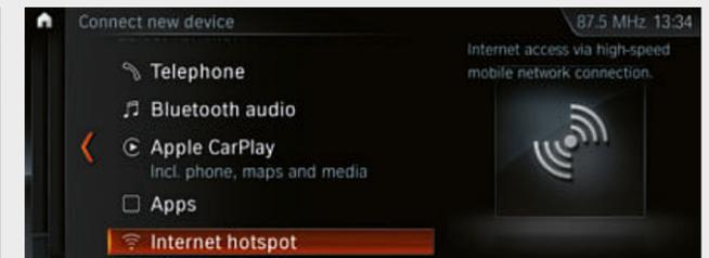
□ The equipment includes a built-in WiFi hotspot<sup>6</sup> using the LTE standard, which allows for a paid Internet connection. The vehicle is connected via the built-in SIM card with a fee-based hotspot plan from a service provider.
