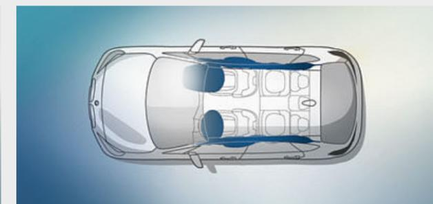
■ The **head airbags** for the first and second seat row complete the vehicle's airbag equipment. With a protective sail that deflects flying shards, they create a highly effective head protection system for the window area that also protects the rear passengers in the event of a side collision.
