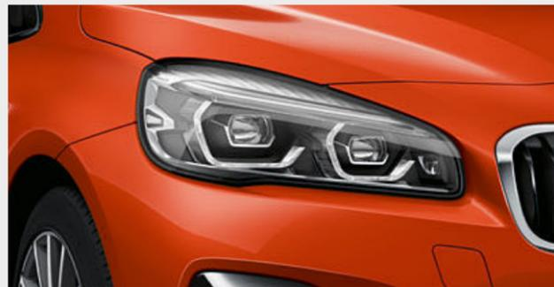
□ The Adaptive LED headlights include low-beam and high-beam headlights and turn indicators with full LED technology. The equipment also features BMW Selective Beam, cornering lights, daytime running lights and Adaptive headlights with variable light control for excellent illumination of the road ahead and better visibility in the dark.
