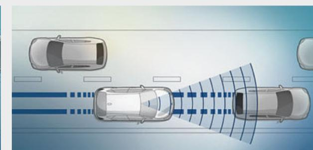
□ **Approach control warning with light city braking function**<sup>1,3</sup> warns of potentially critical situations to help prevent accidents. If there is a risk of collision with a vehicle moving or standing ahead, it provides a two-stage warning and, if necessary, pre-conditions the brakes for increased responsiveness. In case of an emergency, the system initiates braking, ensuring that the collision speed is significantly reduced.
