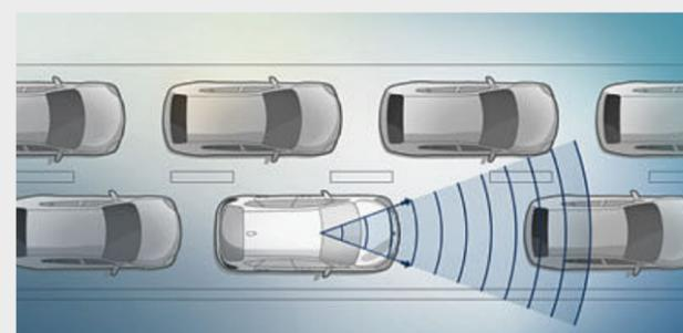
□ **Traffic jam assistant**<sup>4,5</sup> relieves you in monotonous traffic situations on the motorway: At speeds of up to 60 km/h, the system lets the car simply "glide along" with the other cars in dense traffic, making traffic jams less stressful. It automatically maintains the distance from the vehicle ahead and regulates the car's speed down to a standstill – as well as providing steering support.
