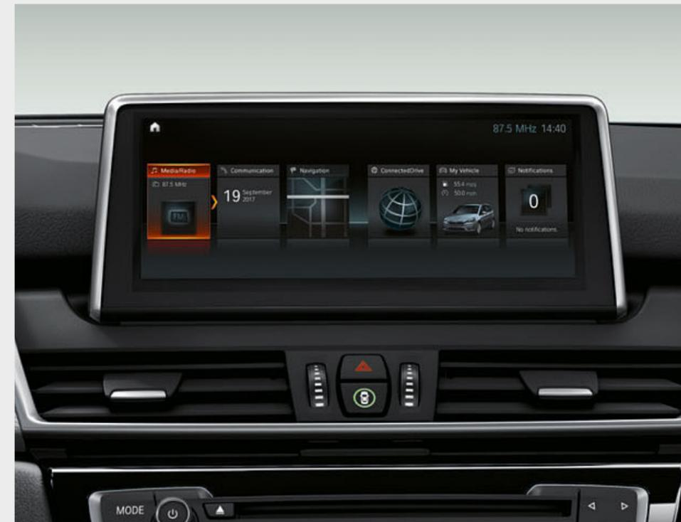
□ Navigation Plus<sup>3</sup> features a BMW Head-Up Display<sup>1</sup>, an iDrive Touch Controller, a built-in 8.8" touch display and an instrument cluster with high-resolution 5.7" TFT display. The system is operated intuitively using either the iDrive Touch Controller, the direct menu control buttons and six or eight functional bookmarks, voice control or the touchscreen with interactive tiles.
