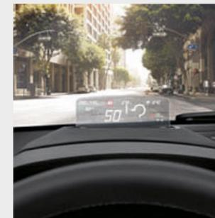
○ The Head-Up Screen puts vehicle information and, in combination with a smartphone interface, navigation information into the driver's line of sight.
