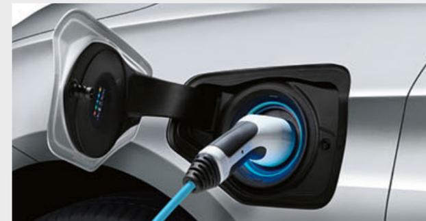
The port for external charging of the high-voltage battery is located behind a flap on the vehicle's front side panel on the left. The charging port is protected from the elements by a special seal. The LED light ring around the port indicates the vehicle's current charge status.
